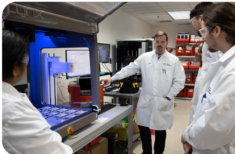
Curtis Walton showcases the Lynx 96VVP, an automated liquid handler widely used at IPI. IPI photo by Sabrina Liu.
