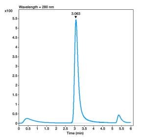
High-performance liquid chromatography-size exclusion chromatography (HPLC-SEC) profile. 5 µg of antibody (1 mg/mL) was analyzed. 1x PBS, pH 7.4 was used as the mobile phase. Protein standards ranging from 15-600 kDa were used for calibration (Sigma, 69385) and Lox1.9 antibody was run as an internal control. Resulting peaks were analyzed using Agilent OpenLab CDS software to determine total peak area and percentage purity.
