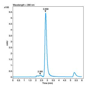
High-performance liquid chromatography-size exclusion chromatography (HPLC-SEC) profile. 5  $\mu$ g of antibody (1 mg/mL) was analyzed. 1x PBS, pH 7.4 was used as the mobile phase. Protein standards ranging from 15-600 kDa were used for calibration (Sigma, 69385) and Lox1.9 antibody was run as an internal control. Resulting peaks were analyzed using Agilent OpenLab CDS software to determine total peak area and percentage purity.
